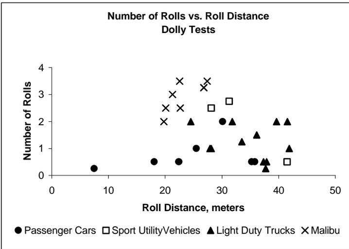
Figure 5. Number of Rolls vs. Roll Distance for All Dolly Tests
