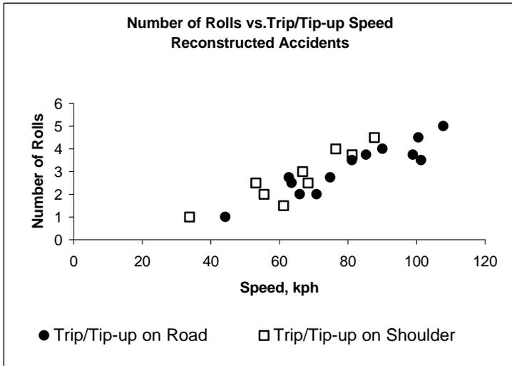
Figure 4. Comparison of location for initiation of rollover for the Reconstructed Accidents
