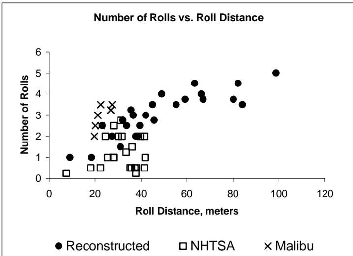
Figure 8. Number of Rolls vs. Roll Distance for Reconstructed Accidents and All Dolly Tests
