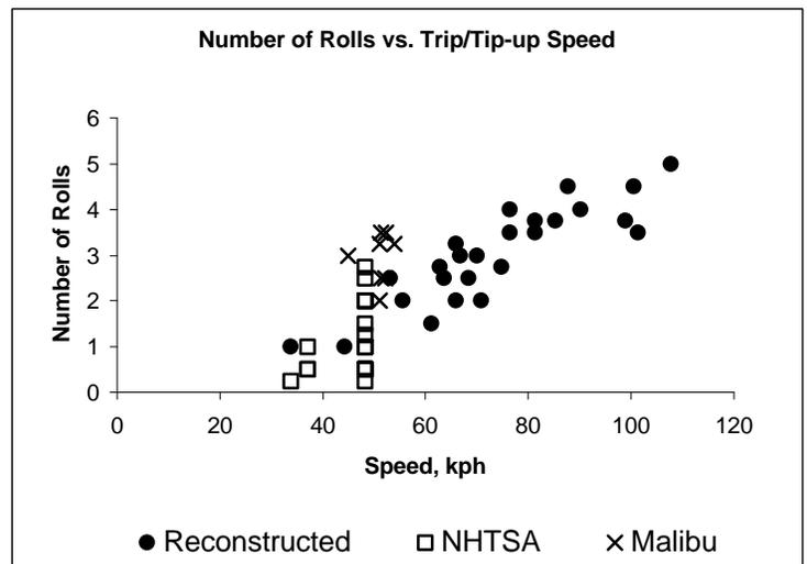
Figure 10. Number of Rolls vs. Trip/tip-up Speed for Reconstructed Accidents and All Dolly Tests
