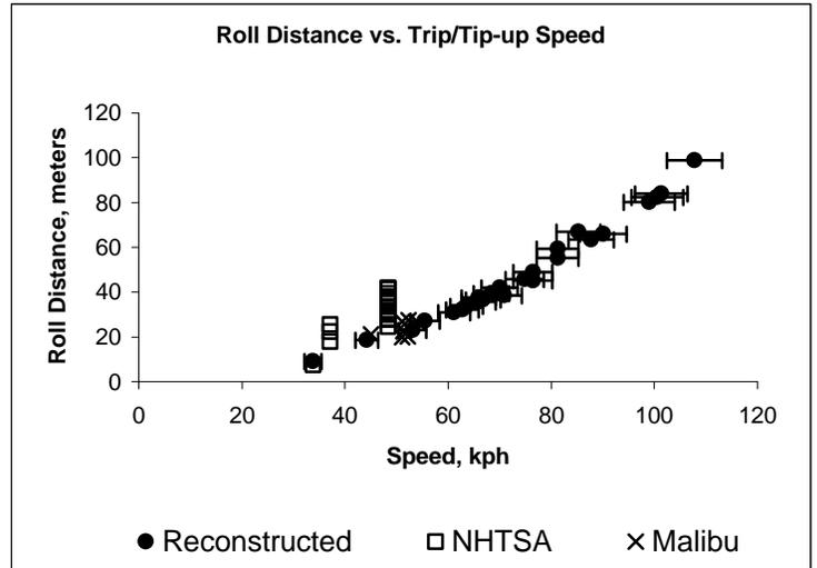
Figure 9. Roll Distance vs. Trip/tip-up Speed for Reconstructed Accidents and All Dolly Tests
