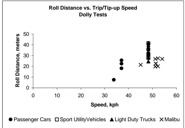
Figure 6. Roll Distance vs. Trip/tip-up Speed for All Dolly Tests
