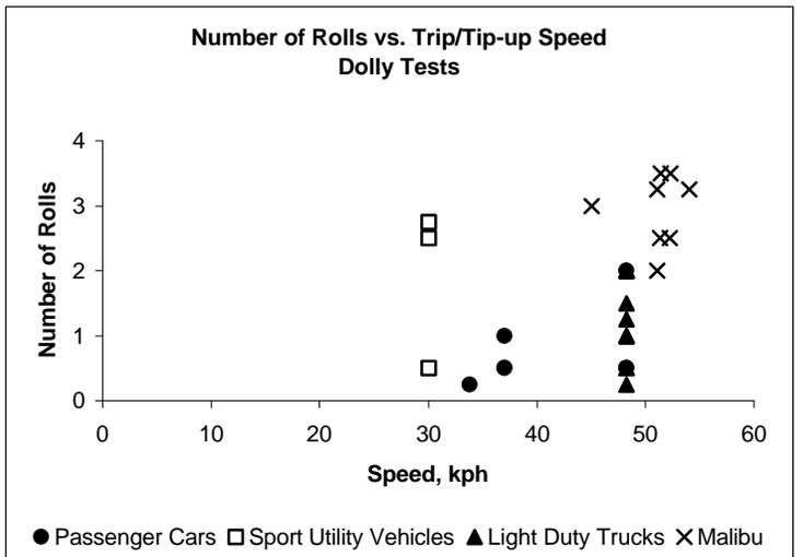
Figure 7. Number of Rolls vs. Trip/tip-up Speed for All Dolly Tests
