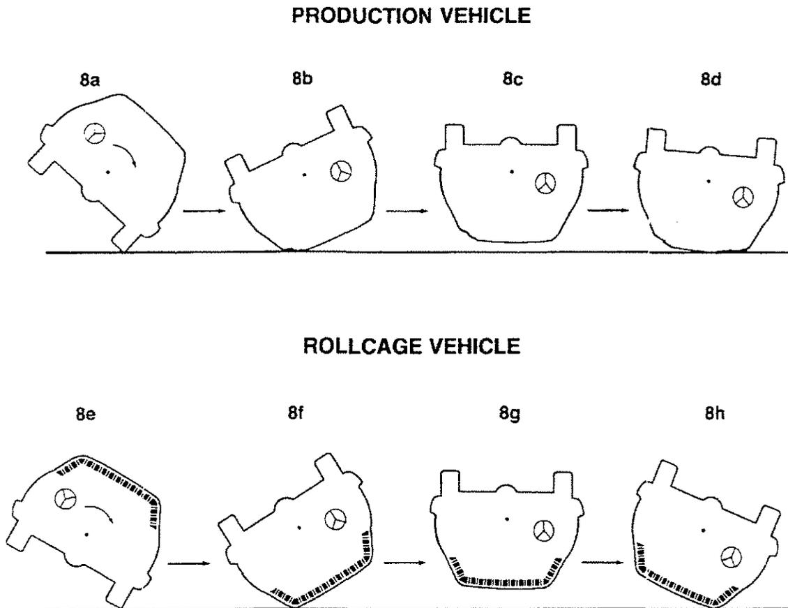
Fig. 8 Kinematic Comparison of Roll Dynamics - Production vs. Rollcage Vehicle
