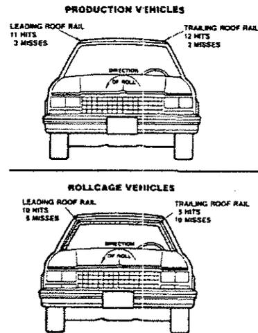
Fig. 7 Comparison of Roof-to-Ground Impacts For Production vs. Rollcage Vehicles
