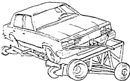
Fig. 3 Vehicle on Dolly Rollover Fixture
