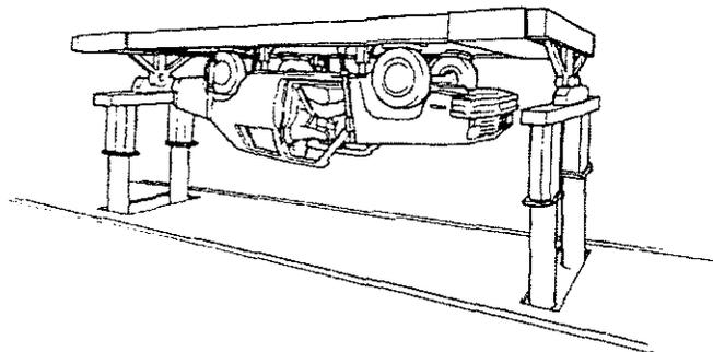
Fig. 1 Occupant Position Tests on FMVSS 301 Vehicle Inversion Device
