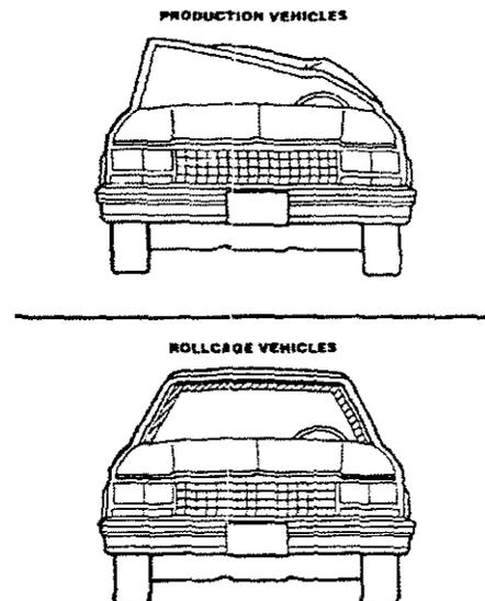
Fig. 15 Roof Crush Pattern of Production and Rollcage Vehicle After 12" Drop Test
