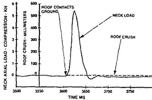
Fig. 12 Roof Crush and Neck Loads vs Time
