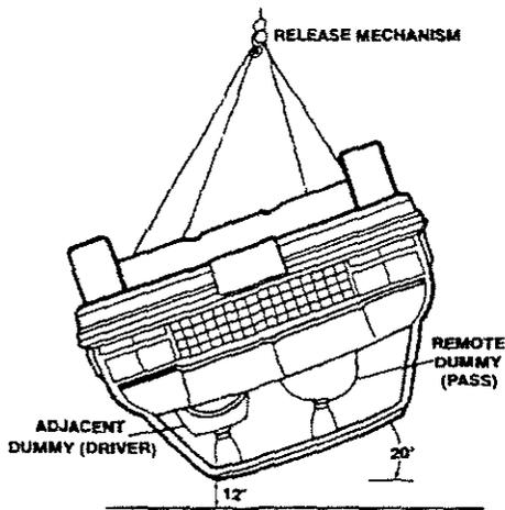
Fig. 14 Vehicle Drop Test
