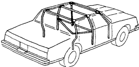
Fig. 4 Vehicle Equipped With Rollcage Structure
