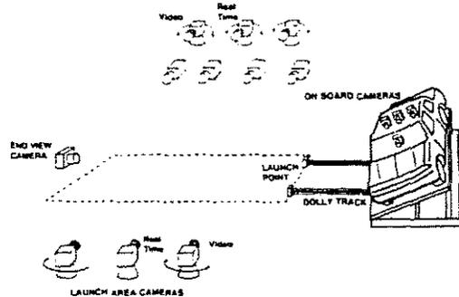
Fig. 5 Dolly Rollover Typical Camera Positions
