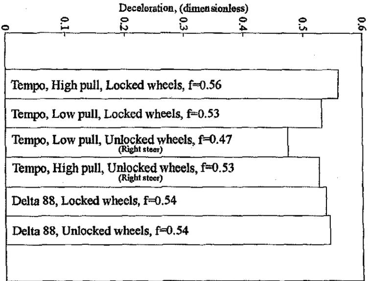
Graph 3: Deceleration rates on constant grass at a 45 degree slip angle. (series one testing)
