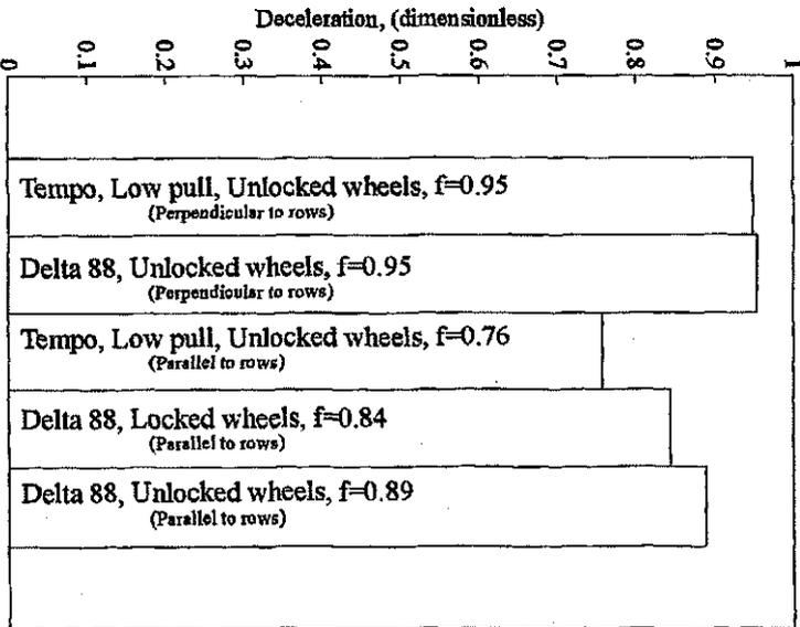
Graph 8: Deceleration rates on harvested corn rows at a 45 degree slip angle. (series one testing)
