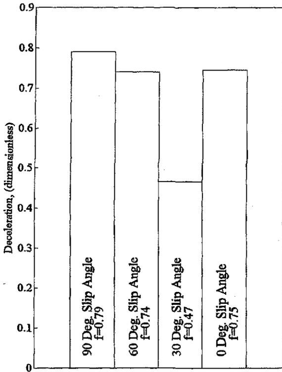
Graph 13: Combined deceleration rates on asphalt for the Chevelle and Vista Cruiser. (series two testing)
