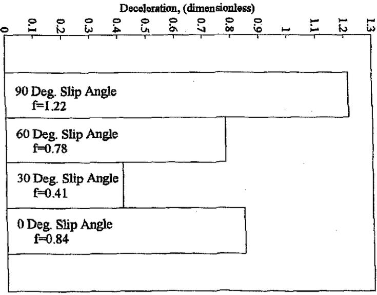
Graph 10: Deceleration rates on black dirt and foliage for the Chevella. (series two testing)
