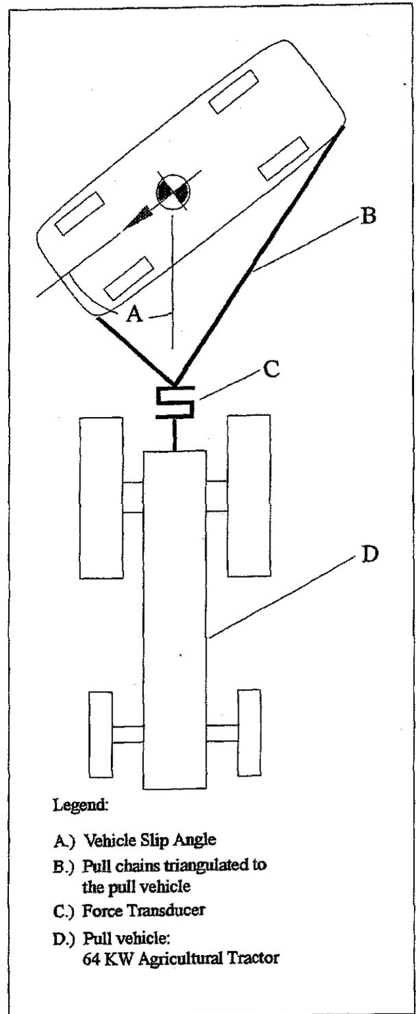
Figure No. 3: Pull configuration setup utilized for the first series of testing.
