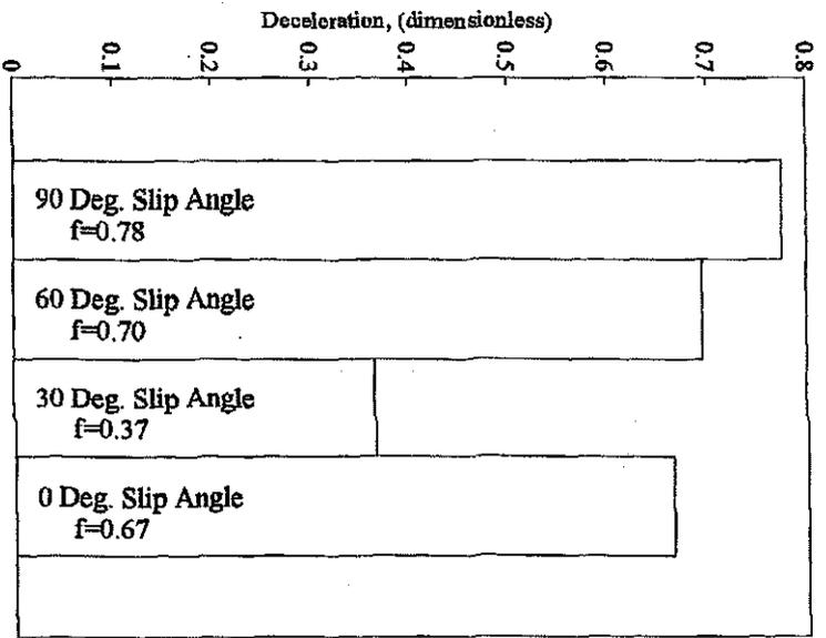
Graph 9: Combined deceleration rates on coastal grass for the Chevella and Vista Cruiser. (series two testing)
