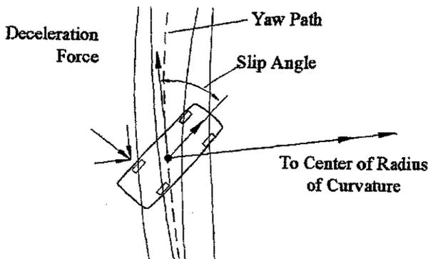
Figure No. 1. Vehicle in side slip yaw path
