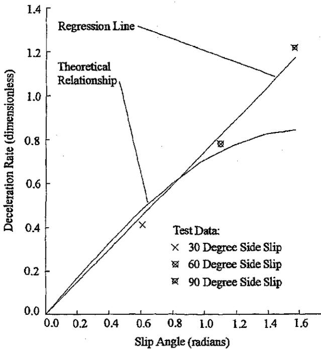
Graph 15: Black Dirt with Foliage Surface Theoretical Relationship and Linear Regression (series two testing).
