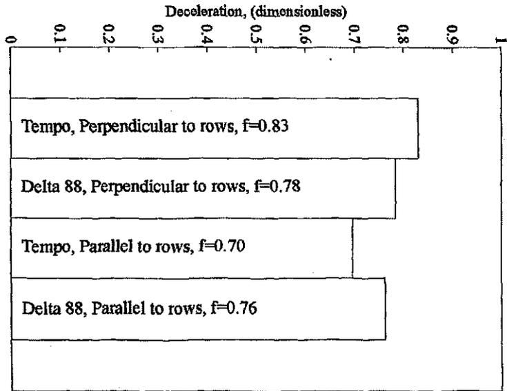
Graph 6: Deceleration rates on harvested corn rows at a 0 degree slip angle. (series one testing)
