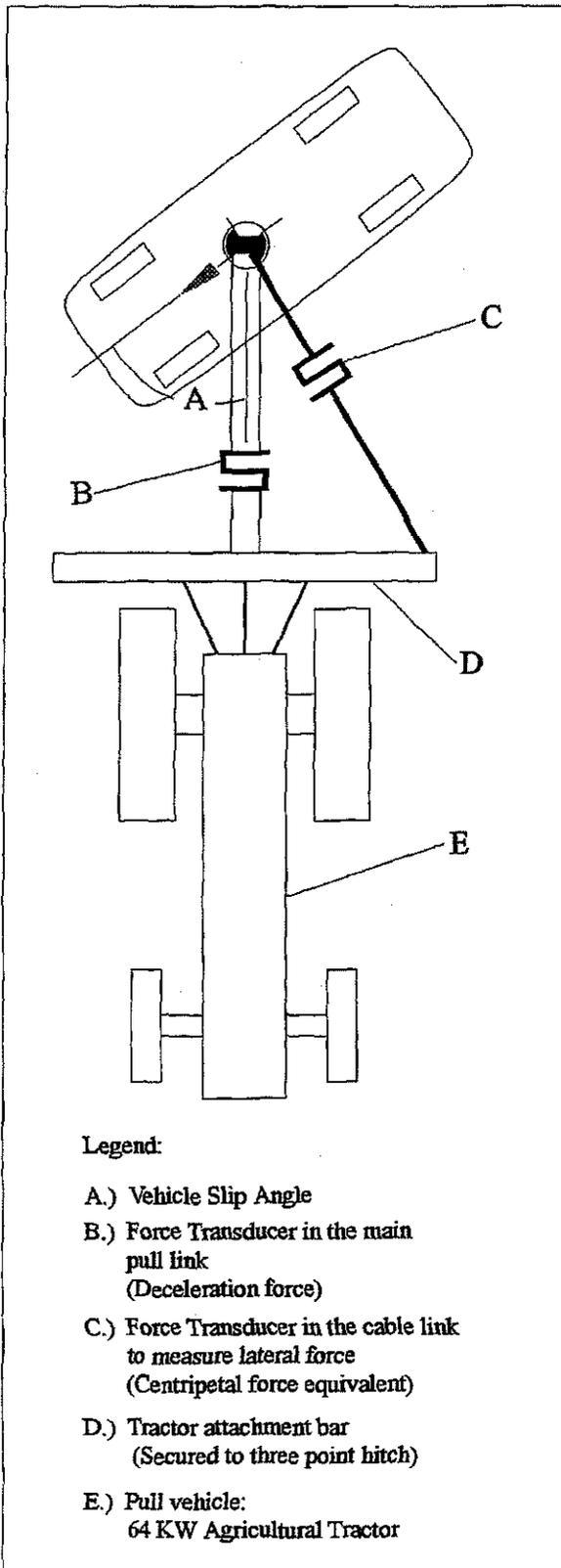
Figure No. 4: Pull configuration setup utilized for the second series of testing.
