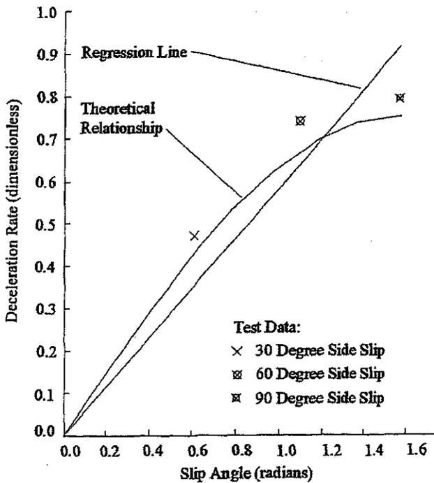
Graph 18: Paved Asphalt Surface, Theoretical Relationship and Linear Regression (series two testing).
