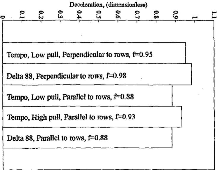
Graph 7: Deceleration rates on harvested corn rows at a 90 degree slip angle. (series one testing)
