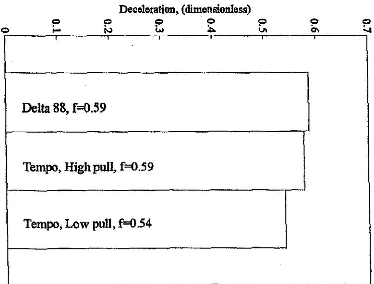
Graph 2: Deceleration rates on constant grass at a 90 degree slip angle. (series one testing)
