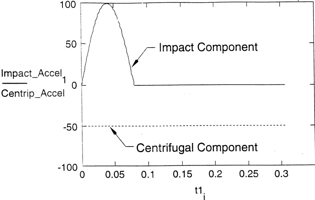
Combined Impact and centrifugal acceleration components in f/s<sup>2</sup>
