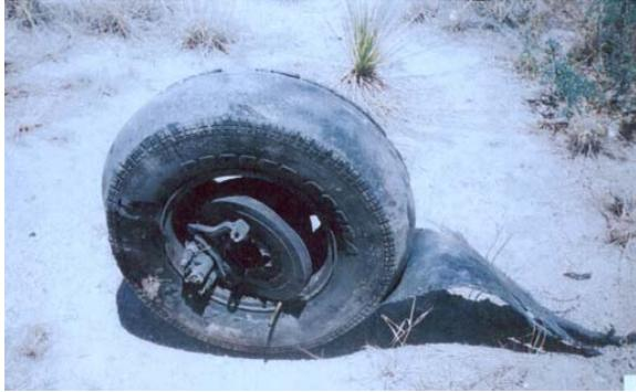
**Figure 6: Photograph of an actual delaminated tire taken at the scene of an accident.**
