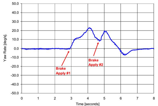
Figure 20. IBT R08 with Pulsed Braking – Yaw Rate
