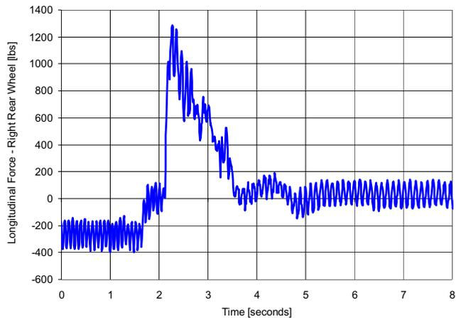
Figure 12. IBT R04 – Longitudinal Force at Right Rear Wheel
