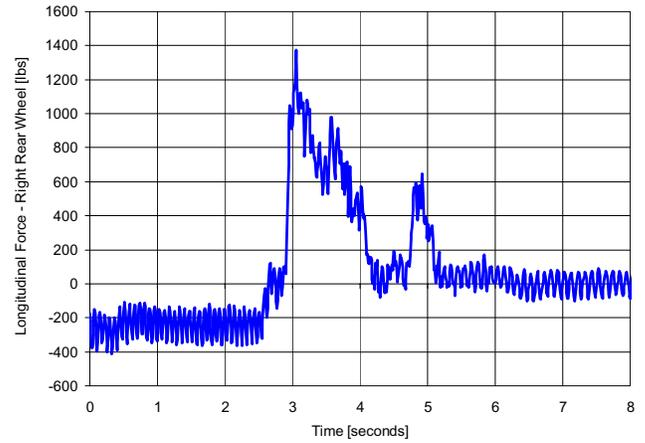
Figure 19. IBT R08 with Pulsed Braking – Right Rear Longitudinal Force
