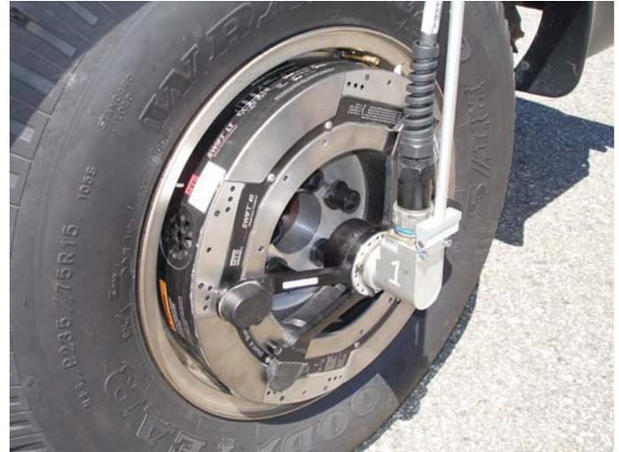
Figure 9. IBT – Wheel Force Transducer at Right Rear Tire Position
