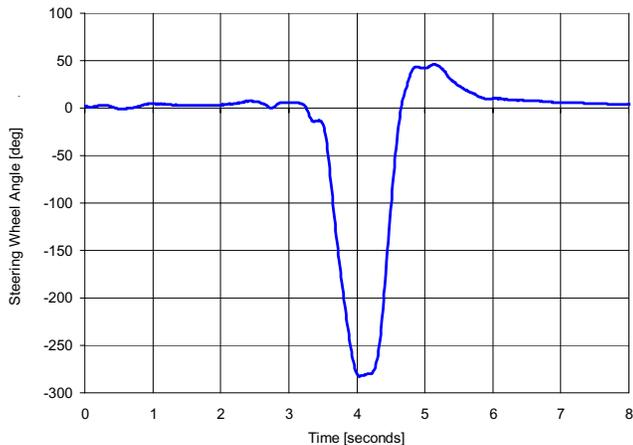
Figure 14. IBT R04 – Steering Wheel Angle
