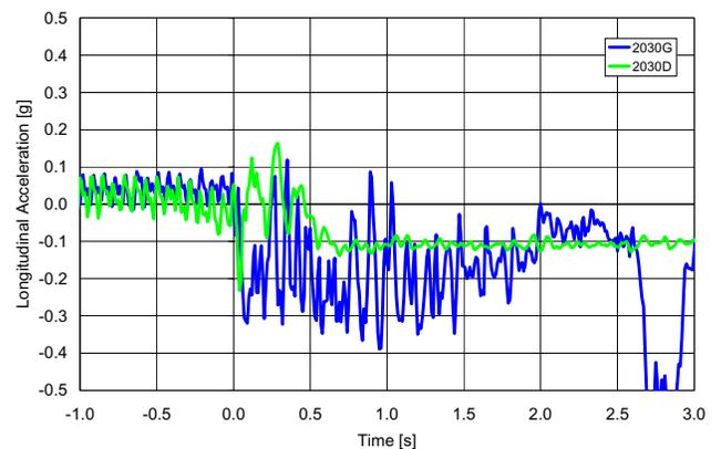
Figure 3. CS1 – Longitudinal Accelerations: 2030D and 2030G
